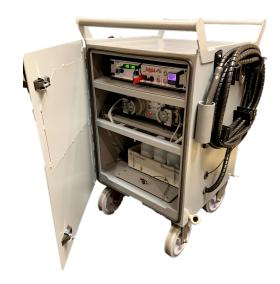
Corrdesa LLC, GA USA, partnered with Dalic, France to produce the ruggedized, mobile Dalistick® system for ZnNi plating repairs directly on aircraft.
